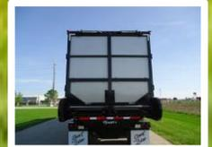
Rear Unload, Dual Hydraulic Motor Drive, 96" Inside Width, 102" Outside Width, 667XH 28,000# Tensile Strength Pintle Apron Chains, 100 Pitch Drive Chains, Vinyl Floor, Air Operated Barn Door Style Rear Doors, Lighting, Options Include: 34', 36' Or 40' Box Lengths, 6' Sides & Optional 2' Extensions, 8' Sides, Folding Front Screen Section, Manual Or Air Cylinder Operated, Grain Hopper, Super Single Tires, Reversing Aprons
